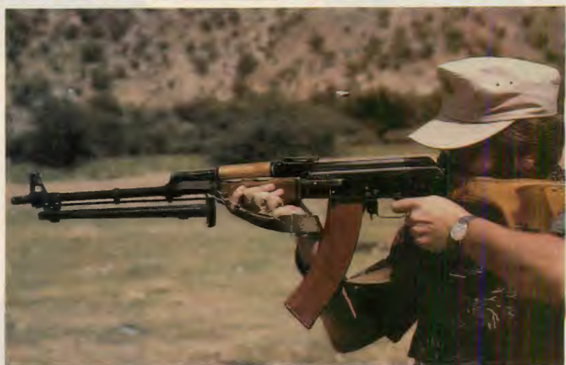
ABOVE: Forward-mounted bipod is more stable than needed by a 12-pound micro-caliber SAW. RIGHT: At 12 pounds fatigue sets in before recoil hurts with new Sov micro-caliber SAW fired from shoulder. BELOW: SOF Foreign Correspondent Jim Coyne shows RPK's "third leg" as 40-round mag drags during prone firing test.
